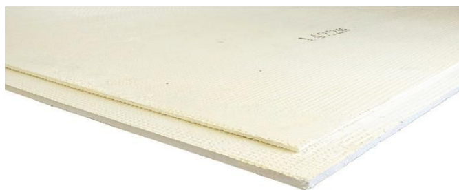
ProPanel backer board offers waterproof performance in a six-pound board. ProPanel consists of high-density expanded polystyrene reinforced on both sides with fiberglass mesh and a polymer cement coating.
